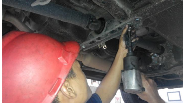
Gambar 19. Melepas mounting propeller
