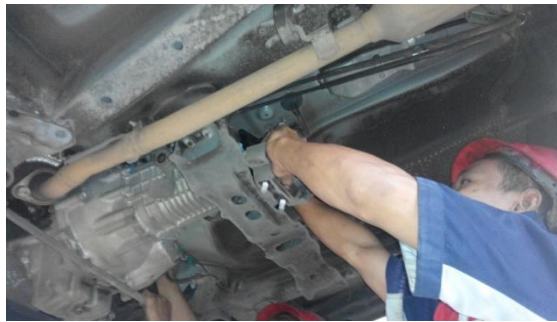
Gambar 23. Melepas mounting transmisi
