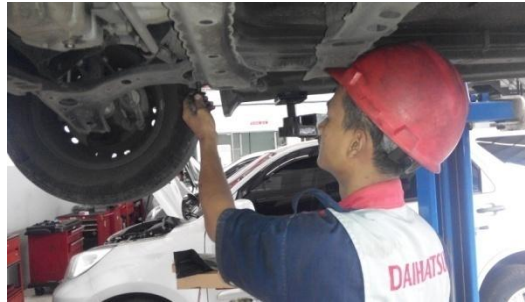
Gambar 16. Melepas under cover mesin
